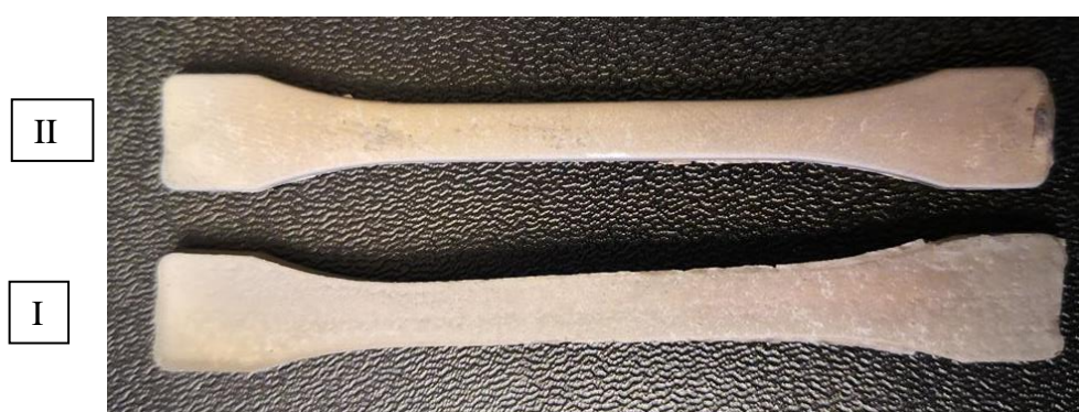
Rysunek 6. Próbkki po spiekaniu, I-1350°C, II-1300° Figure 6. Samples after sintering, I-1350°C, II-1300°
