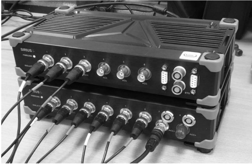
Fig 3. Sirius data acquisition module
