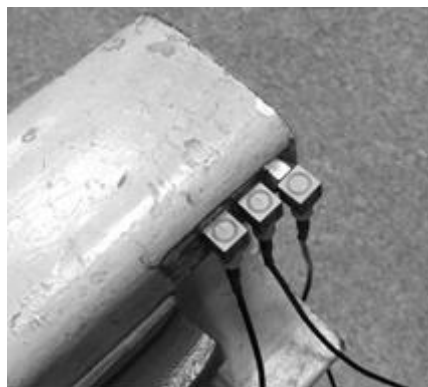
Fig 4. Endevco accelerometers are mounted on the cleaned side wall of the rail head, where successively (from the left) they are mounted on cyanoacrylate glue, beeswax and the factory accessory of sensors - a magnet.
