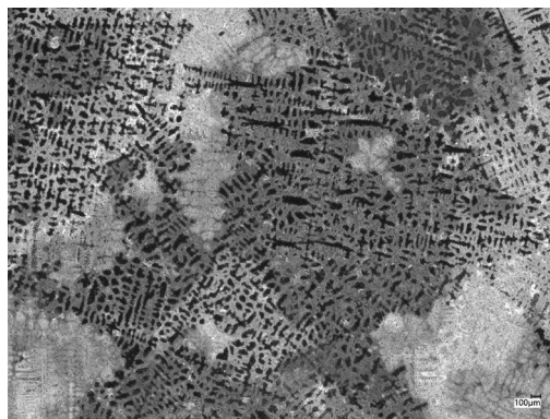
Figure 8. Microstructure of the CuTi4 ingot from the central area. Light microscopy, etched sample
