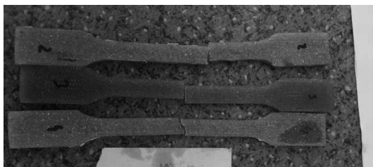
Figure 16. Composite with larch 15%
