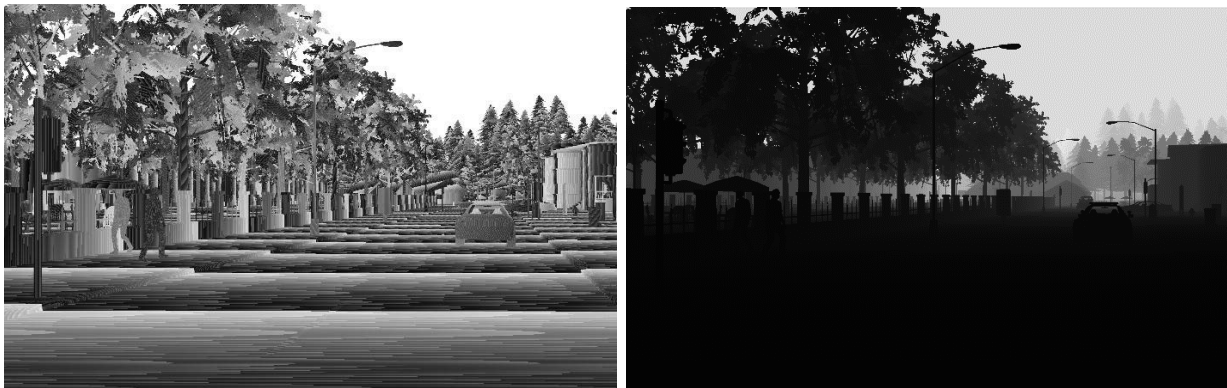
Figure 2. The left image shows the output depth map from the CARLA simulator, while the right shows the normalised image.
