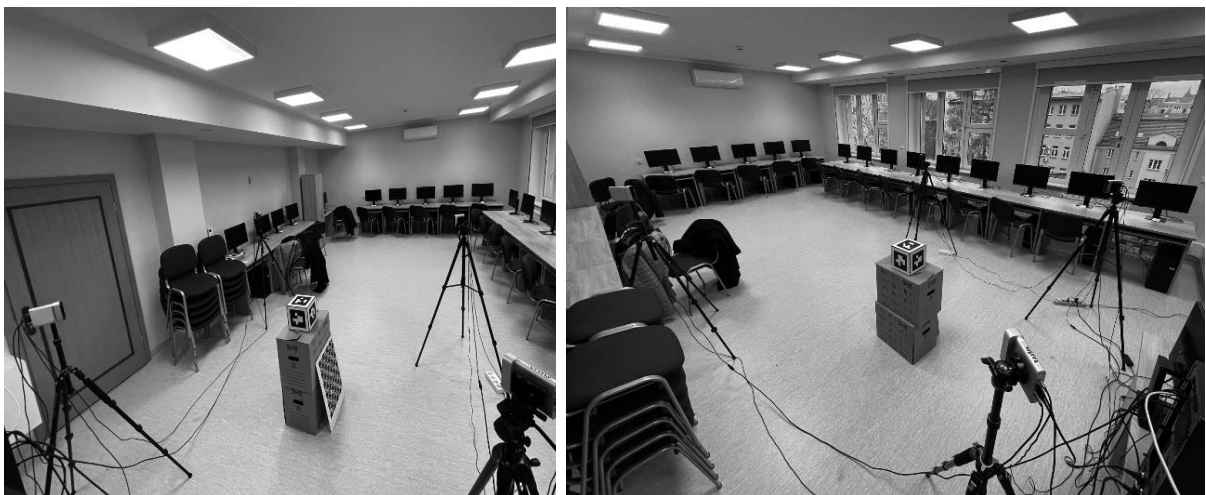
Figure 3. Configuration of Azure Kinect DK sensors utilized for 360-degree 3D point cloud acquisition, featuring a visible ArUco cube used for spatial calibration.
