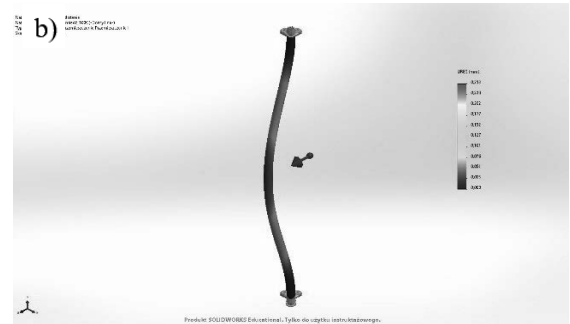
Fig. 6. Displacement of copper cable subjected temperature to: a) 30°C, b) 100°C, c) 140°C.
