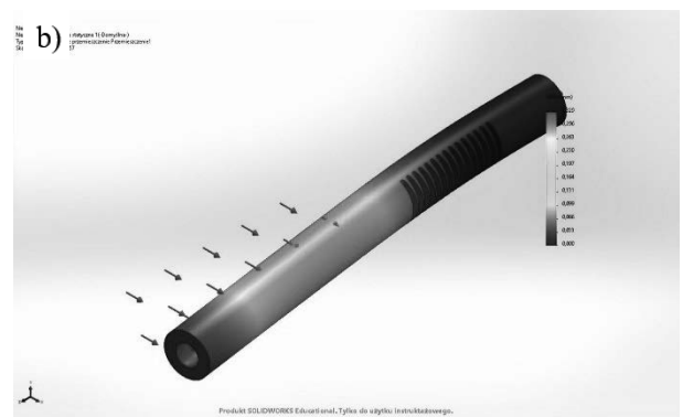
Fig. 6. Under a force of 500N on the strip in the direction of the notches, the results are shown: a) Tension, b) Displacement, c) Deformation.
