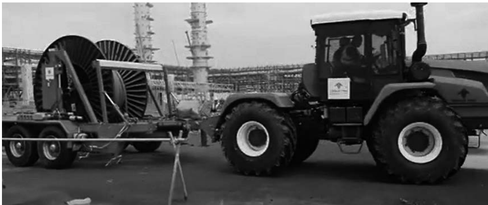
Figure 2: Cable Transport Trailer and Transport Vehicle
