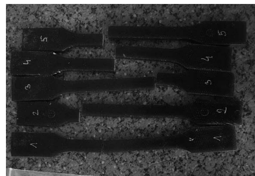
Figure 17. Composite with alder 5%
