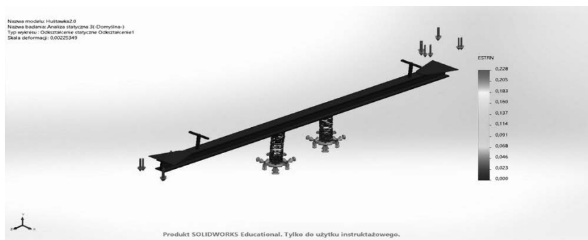
Fig. 10 The result of the deformation for the applied forces 560 N i 400 N.
