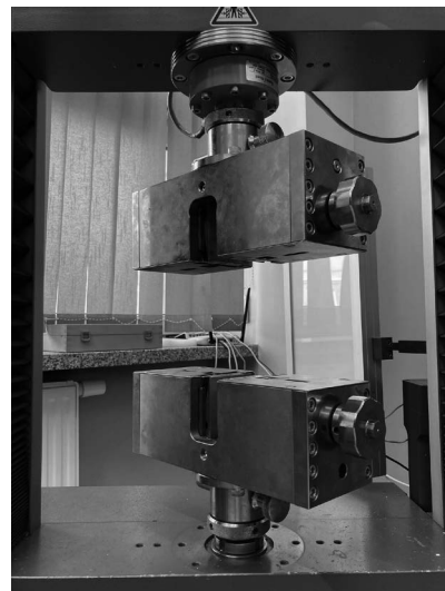
Figure 4. Holders for conducting a static tensile test mounted on the Zwick/Roell Z020 device.
