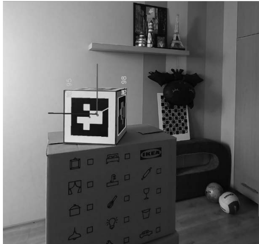
Figure 4. Example RGB image with the highlighted ArUco markers detected on the calibration cube
