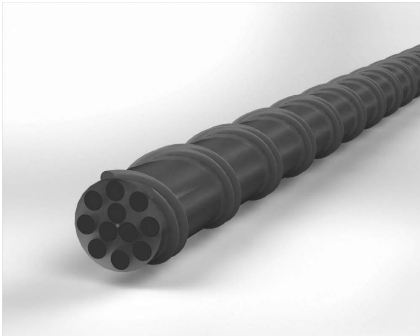
Figure 3. 3D model of composite rod with integrated OS sensor. 1 - fiber optic sensor, 2 - fiberglass, 3 - resin, 4 - double helical glass fiber "notch".
