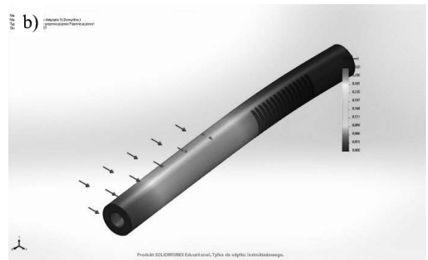
Fig. 5. When a force of 500N is applied to the strip against the notches, the results are shown: a) Tension, b) Displacement, c) Deformation.
