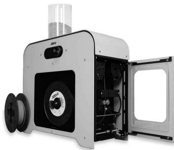
Figure 2. a) 3D Evo Composer 350 device [10], b) processed granules from bottle caps
