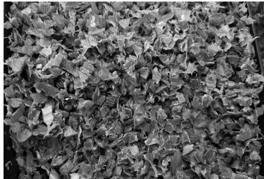
Figure 2. a) 3D Evo Composer 350 device [10], b) processed granules from bottle caps
