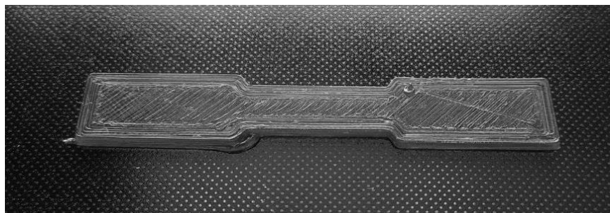
Figure 14 - Printed sample for tensile research
