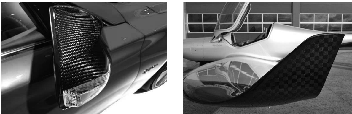
Obr. 3 Použitie CFRP v leteckom a automobilovom priemysle Figure 3. Application of CFRP in aerospace and automotive industry
