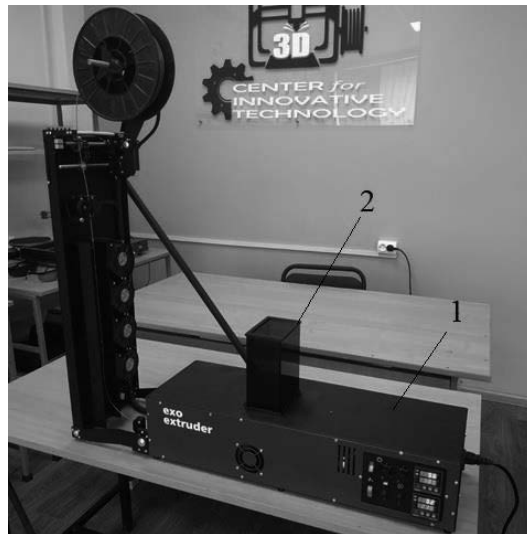
Figure 2 - Extruder for the manufacture of a filament with a metal filler for 3D printing: 1 - the housing with the heating system; 2 - the loading unit
