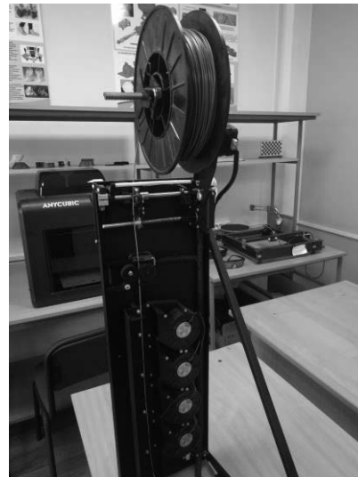
Figure 4 - Cooling and winding systems for filament
