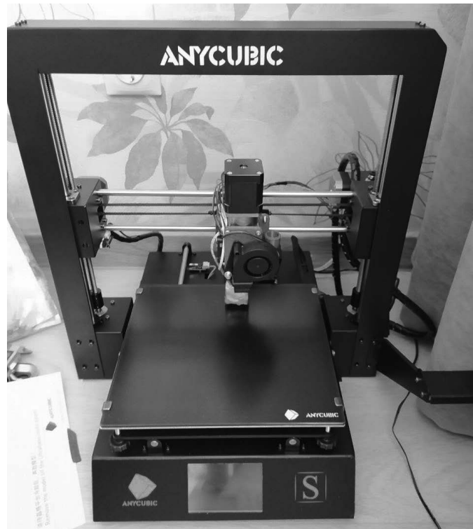
Figure 8 - General view of the Anycubic Mega S 3D printer with installed extruder
