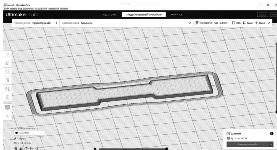
Figure 9 - Layer-by-layer breakdown of the sample in the form of a scapula
