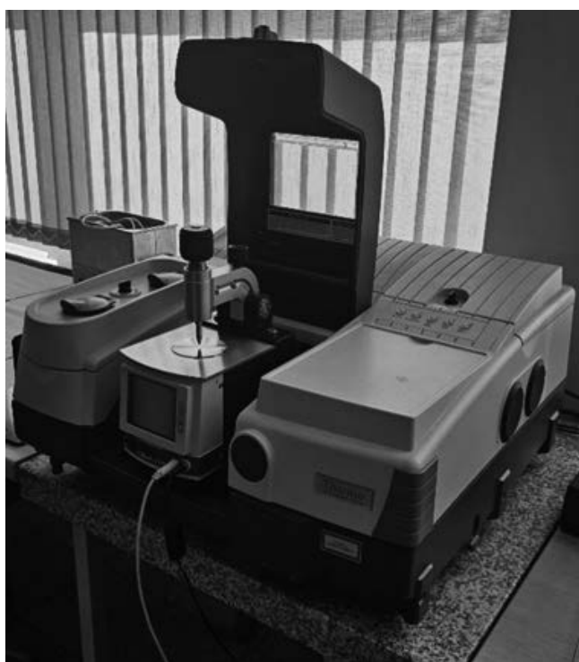
Fig. 1. Spectroscopy system "Thermo Scientific" with the "Gladi ATR"
