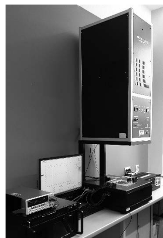
Figure 2. System for measuring current-voltage characteristics from PV Test Solutions Tadeusz Żdanowicz
