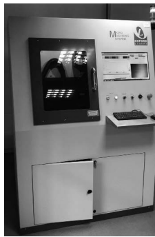
Figure 2. A-355 picosecond laser system and machine parameters (specification).
