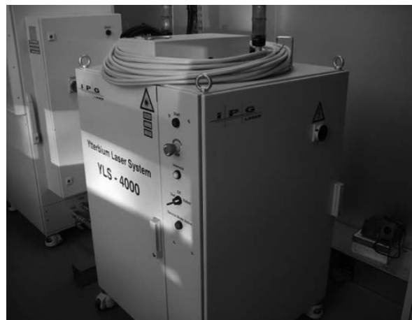
Fig. 1 IPG YLS - 4000 laser source.
