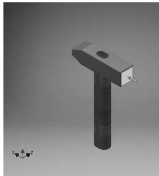
Figure 3. Point of application force
