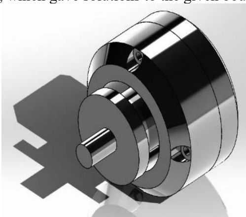
Figure 2. Geometric model of the gearbox cushion
