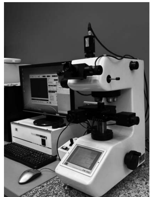
Figure 3. Future-Tech ARS-9000 microhardness tester
