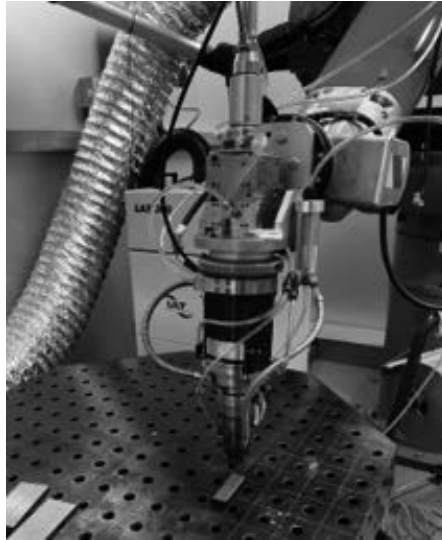
Figure 1. View of robotic LMD surfacing station used for sample surfacing
