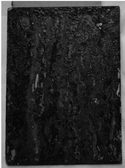
Figure 1. Sample after 360h in salt chamber
