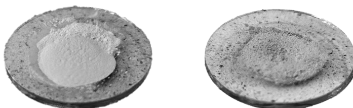
Figure 4. Images of intermediate product SnHydOx_Agm (left) and resulting nanopowder SnOx_Agm (right)
