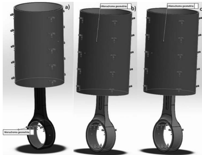
Fig. 8. View of places with fixed translation: a) model with deep bowl, b) model with deep bowl with cooling galleries, c) model with flat bowl
