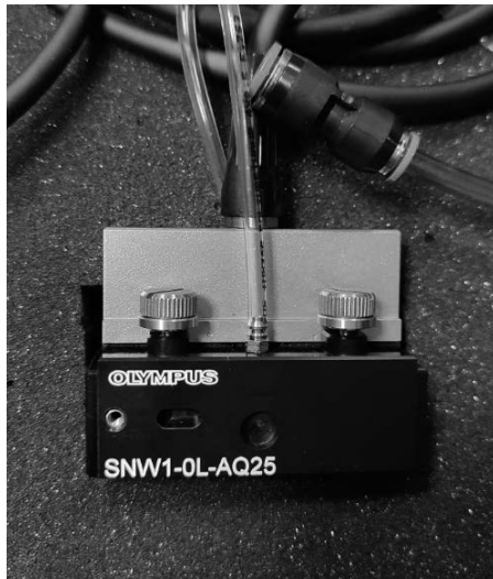
Figure 4. The 3.5L64-NW1 head used in the study, along with the SNW1-0L-AQ25 wedge
