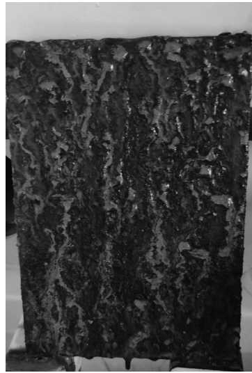
Figure 2. Sample after 720h in salt chamber
