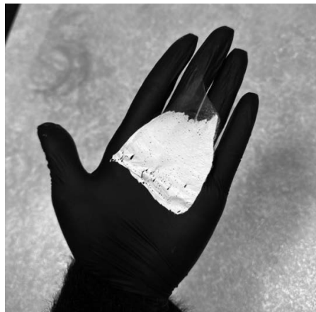
Figure. 2. PVP fibers produced in the electrospinning process.
