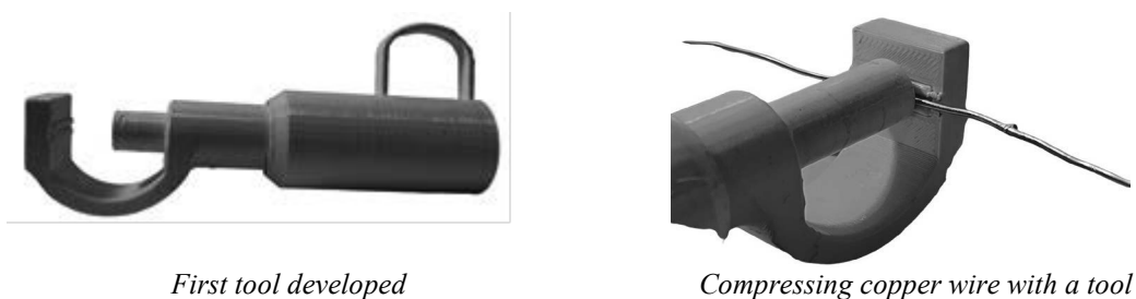
Figure 2: The solid view of tool and its application
