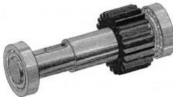
Obr. 1 Valivé uloženia: hriadel' podopretý dvoma ložiskami [1] Figure 1. Rolling bearings, shaft supported by two bearings [1]
