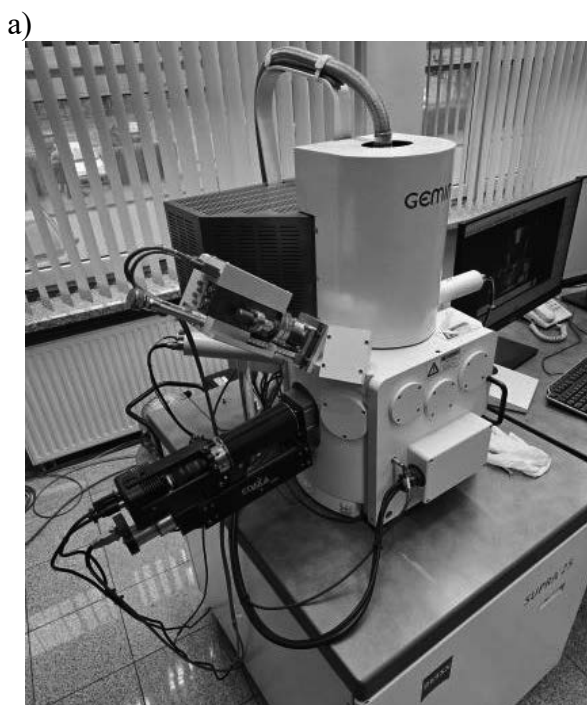
Figure 1. Zeiss Supra 35 scanning electron microscope (a) measuring table with samples (b)
