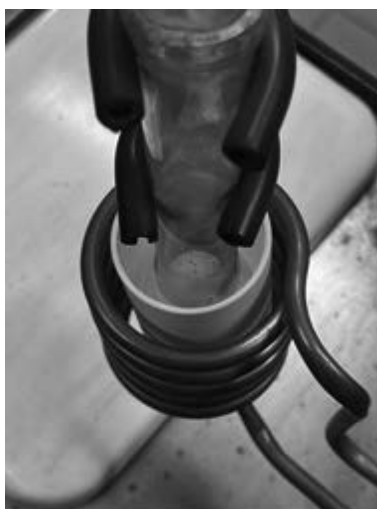
Figure 1. Induction melting of pure elements in a ceramic crucible
