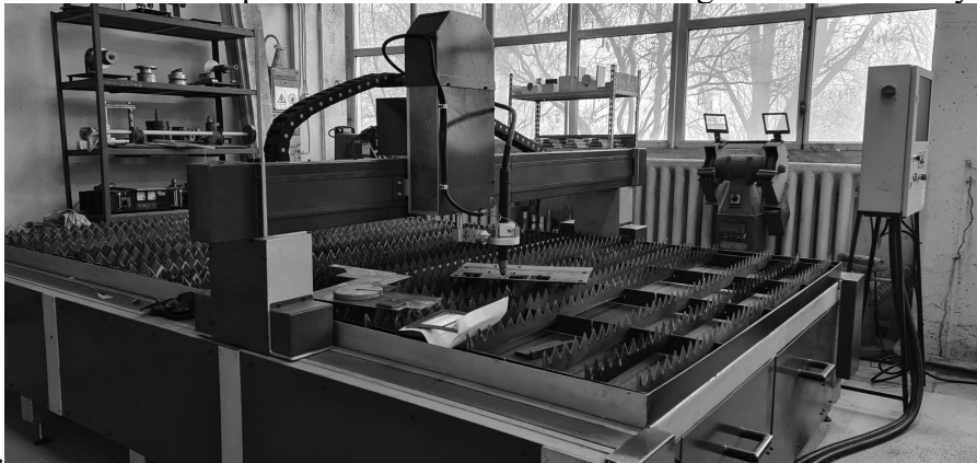
Figure 1. CNC plasma jet cutting machine with 3 axes (University of Petrosani)
