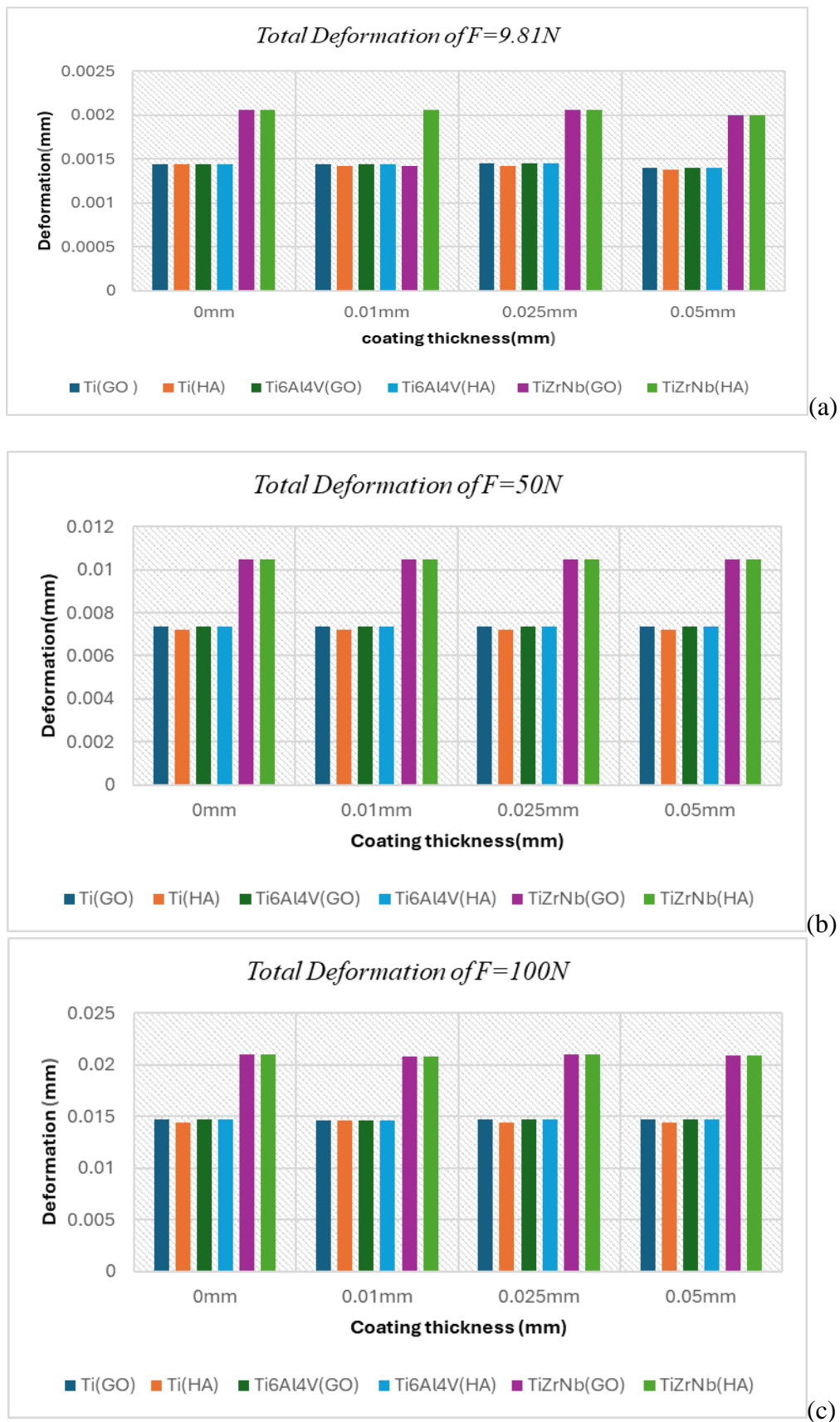
Figure 2(a-c) a. Ti alloy deformation with application of 9.81N b. Ti alloy deformation with the application of 50N c. Ti alloy deformation with the application of 100N.
