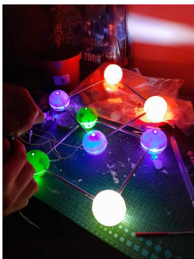
Fig. 3. Optimisation of material colour and type of filament material as a function of light scattering quality
