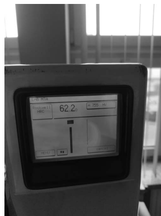
Fig. 2. Example of Rockwell hardness result for a sample of C45 steel
