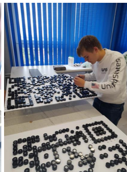
Fig. 5. Stage of bonding samples to glass plates using UV-curable adhesive
