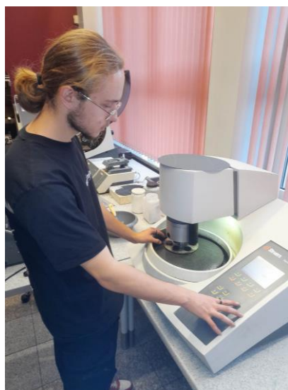
Fig. 4. Preparation of additional samples using Tegramin's integrated specimen mover, automated process control
