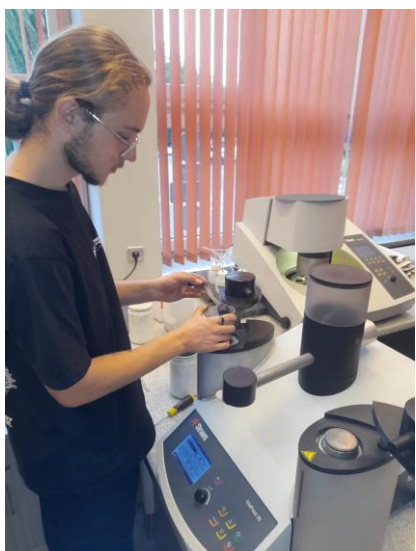
Fig. 3. Preparation of additional samples using CitoPress is a high-performance hot mounting press
