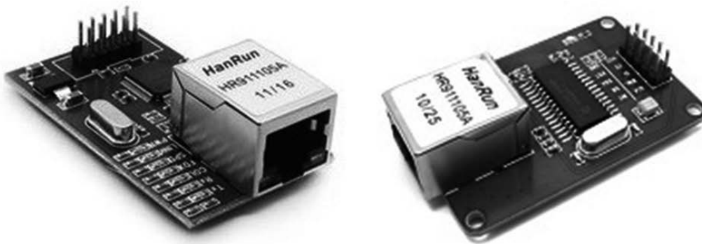
Figure 6. Network extension board
