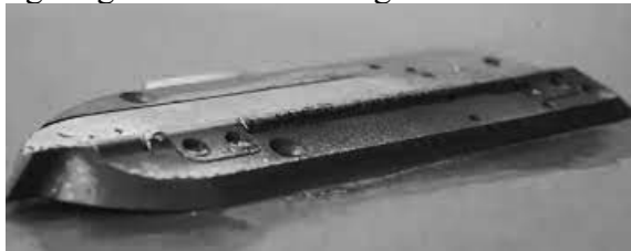
Figure 1. Smart Vortex Generators in closed position
