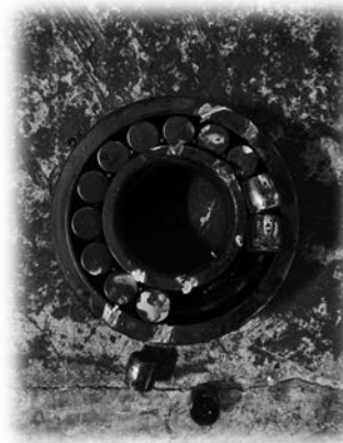
Figure 7. Damaged bearing cage
