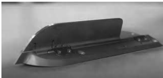
Figure 2. Smart Vortex Generators in open position
