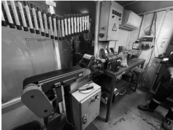
Figure 1. Extruder Strip Sample Production Machine of NEXANS Company
