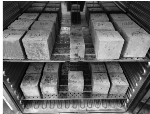
b) samples 10x10x10cm curing in air 35°C
