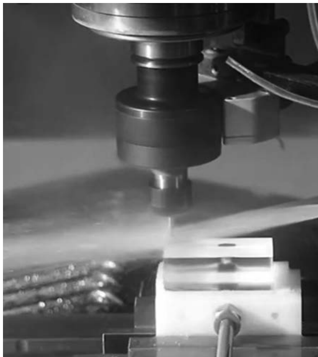
Figure 3 Ultrasonic grinding of quartz glass
