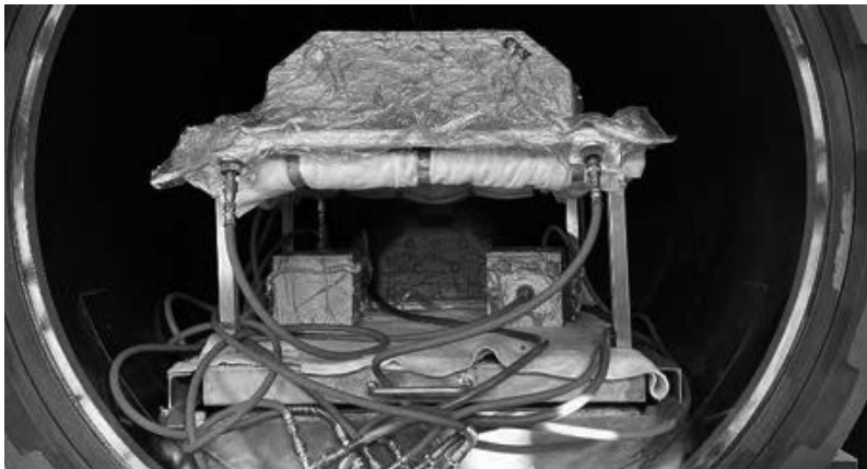
Fig. 6. Components prepared for heat curing in an autoclave
