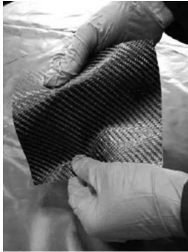
Fig. 5 Preimpregnate pre-soaked in resin.
