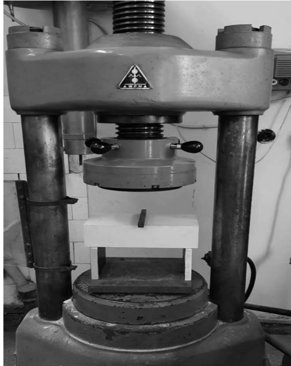
Figure 2. Compression testing of brick with hydraulic press
