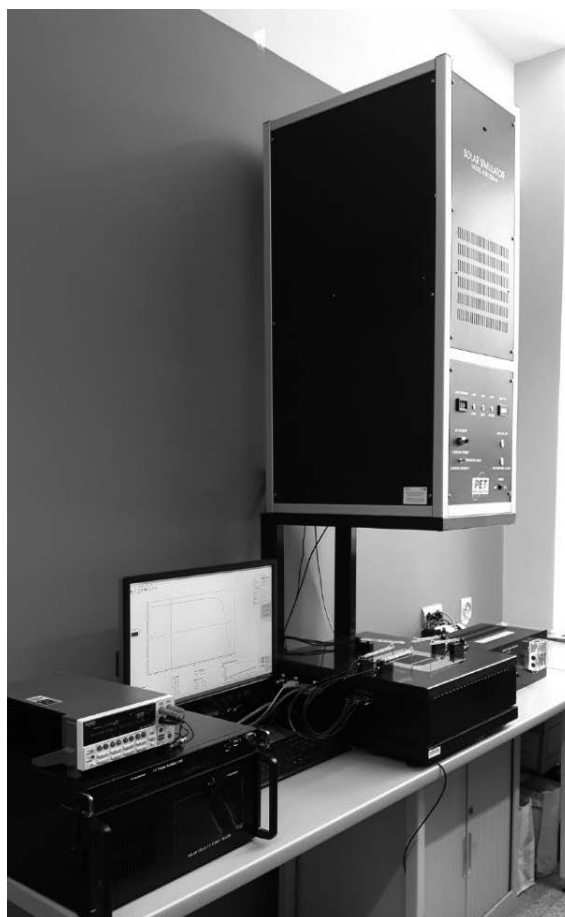
Figure 4. System for measuring the current-voltage characteristics of solar cells equipped with an SS150AAA solar radiation simulator
