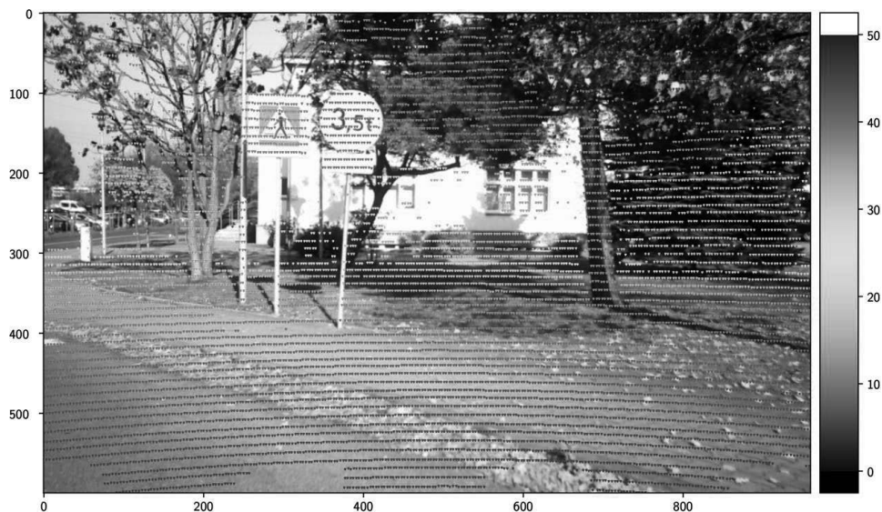
Figure 1. A frame captured from the camera image with the corresponding points from the LIDAR projected onto it. The LIDAR points are overlaid on the image in a way that aligns with the camera's perspective, providing a combined view of the scene.
