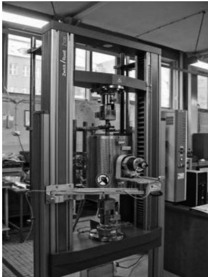
Figure.2 Zwick / Roel Z100 machine[5].
