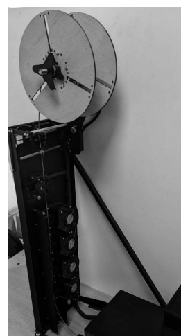
Figure 5 - Systems of cooling and winding of polymer thread
