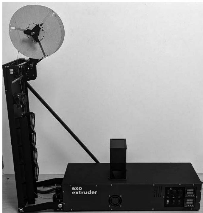
Figure 3 – Extrusion machine: 1 - housing with a heating system; 2 - loading block
