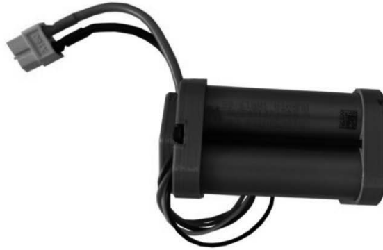
Figure 2. Battery pack made of Sony US18650VTC4 cells
