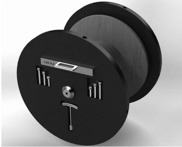
Figure 8: Final render image of mobile winding reel
