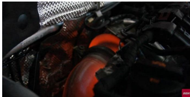
Fig. 1. High efficient turbo charger during work – heated up to glowing temperature [11].
