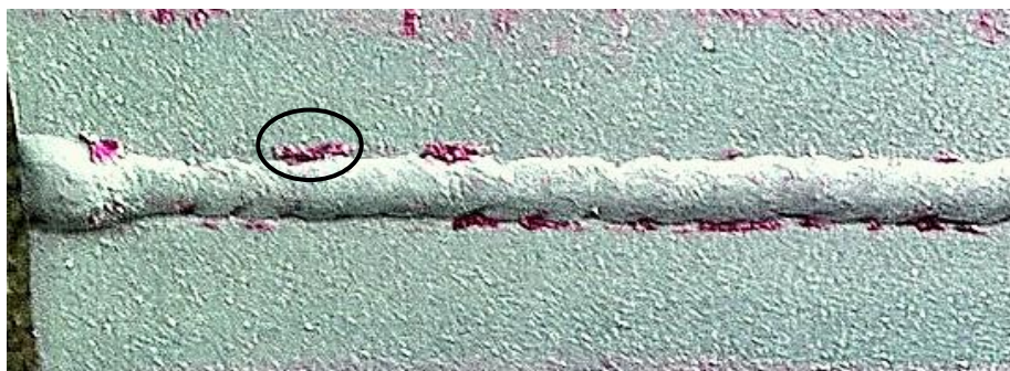
Rysunek 11. Wskazania na grani spoiny Figure 11. Indications on the welding root
